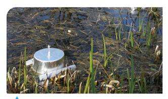
Greenhouse gases have been intensively sampled in 250 ponds in the **PONDERFUL** project. Such floating chambers catch the bubbles of methane emitted in the anoxic sediments of the pond. © HES-SO
