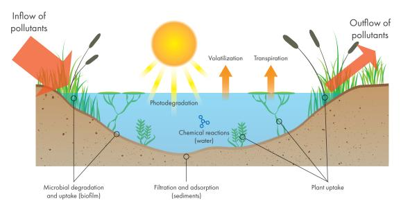
Fig. 11 - Purification in ponds is linked to the cumulative effect of various processes: filtration, chemical degradation (e.g photode-gradation, hydrolysis), microbial degradation, volatilisation, adsorption on sediments, vegetation and organic matter, and plant and microbial uptake.
