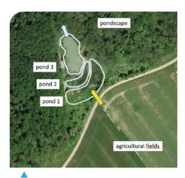
The polluted water (yellow arrow) is intercepted by a first well-vegetated pond, before flowing into a second and later a third pond. The purified water (blue arrow) then flows downstream towards the pondscape where it will feed other waterbodies.
