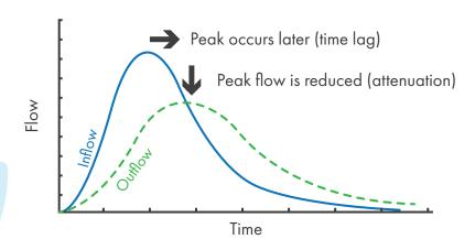
Fig. 9 - Ponds can significantly reduce and delay peak flows during flood events.
