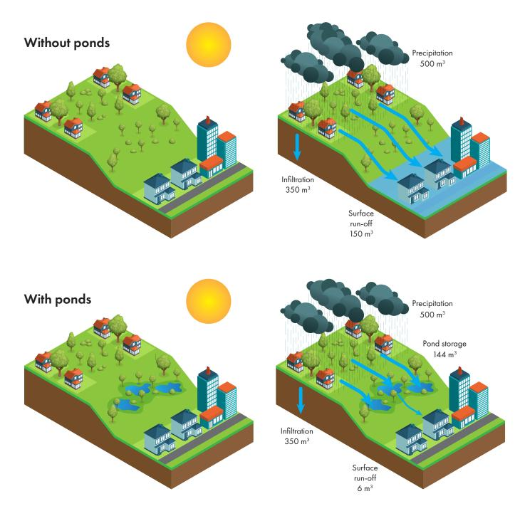
**Fig. 10 -** Simplified illustration of the benefit provided by a small pondscape situated in the catchment of an urban area during a storm event. The upper figure presents the situation without the pondscape, before (left) and after (right) a storm event. The lower figure presents the same situation, but with the benefit of the pondscape of three ponds of 300 m<sup>2</sup> with a drawdown zone that is able to store 144 m<sup>3</sup> of rainwater, reducing flood risk.
