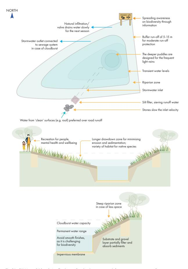
Fig. 26 - CLIMA-pond Urban design. This design is for urban locations primarily focusing on water storage, pollution interception, minimising greenhouse gas production and providing biodiversity benefits where possible. © Amphi International ApS
